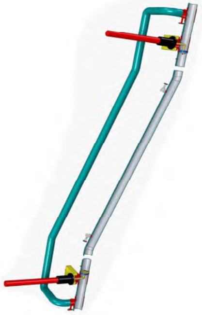
Fig. Cold-Cutting of Header Pipe.
