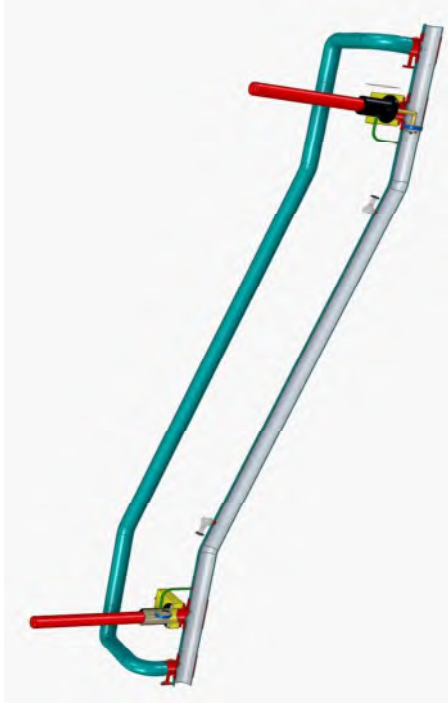
Fig. Insertion of Downstream Stopple Plug into Pipeline.
