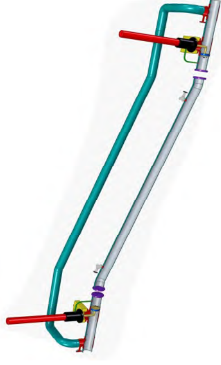
Fig. Welding of Dish Ends into the Live and Dead Section , Pressure Equalization for Stopple Plug Retrieval.
